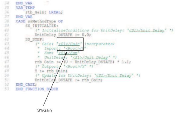
2 In the HTML report window, click a link to highlight the corresponding source block. For example, in the HTML report shown in the previous figure, you click the hyperlink for the Gain block (highlighted) to view that block in the model. Clicking the hyperlink locates and displays the corresponding block in the model editor window. You can use the same method to trace other block from the HTML report.
