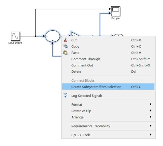
Optionally, rename In1 and Out1 to U and Y respectively. This operation results in a subsystem like the following figure:
