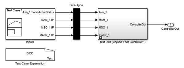
**c** Open the Inputs block in the test harness model. The Inputs block is a Signal Builder block that can have one or more signal groups.
