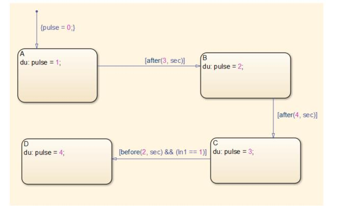
You can map states and transitions in the chart to the generated code. For instance, the transition from state B to C appears as:
