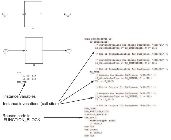
4 Examine the generated Structured Text code. The code defines FUNCTION\_BLOCK S1 once.
