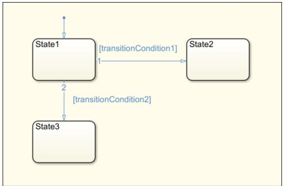
Some advanced Stateflow features on page 3-19 are not supported because of inherent restrictions in Ladder Diagram semantics. You can use the function plccheckforladder to check if the chart has the required properties. You can also use the function plcprepareforladder to change certain chart properties so that the chart is ready for Ladder Diagram code generation.
