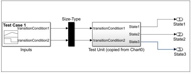
You can also create tests by using other blocks from the Simulink library. However, you must ensure that the inputs to the chart are Boolean.
